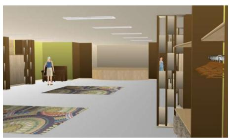
One of the key aspects of the renovation involves unique wall partitions. We plan to adorn the walls with spaced wood beams, reaching from the floor to the ceiling, creating a distinctive "wall booth" design. These booths will not only match the overall architecture of the building but give the room character and serve as practical storage spaces for chairs, tables, and portable partitions.
